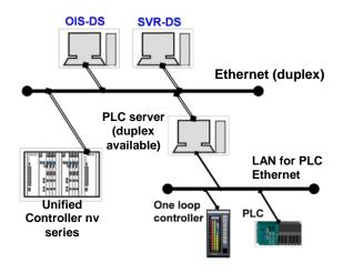
(1) To connect through PLC server PLCs can be connected through PLC server using Ethernet as the connection interface. Connectable PLCs includes MELSEC-A series and SYSMAC CS/J series. (For other models, please contact us.)
